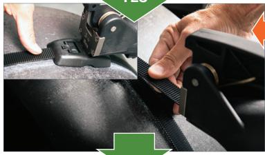
NOTE – The Mountz torque wrench is factory set to the correct torque requirement for the specified product being used. The set torque is marked on the wrench.
