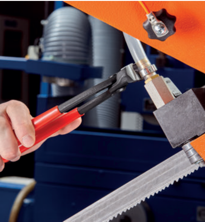
Sealing the fluid hose on the connecting piece using the side press nib
